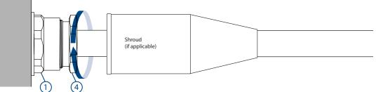
**NOTE:** Support the cable to prevent it twisting. To aid wiring inside the enclosure, it may be necessary to strip the inner sheath prior to bringing the cable through the gland.
